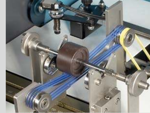
Balancing of permanent magnet armatures with 3 drive belts (Pasio 5)
