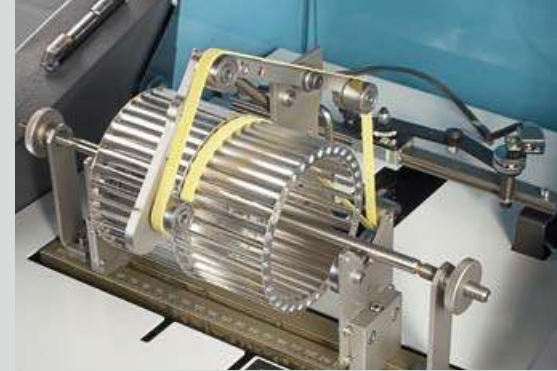
Belt drive from above for balancing of radial fans (Pasio 5)
