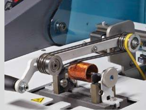
Tangential drive for very lightweight rotors such as non-ferrous armatures (Pasio 05)
