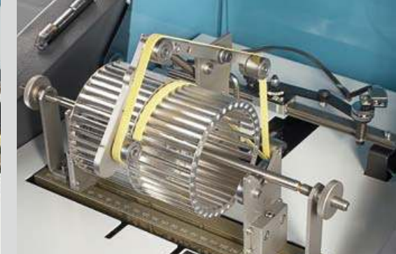
Belt drive from above for balancing of radial fans (Pasio 5)
